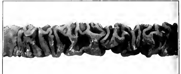
Portion of an 18-ft. Length of Steel Pipe Which Crushed to a Length of Six Feet Without Failure
